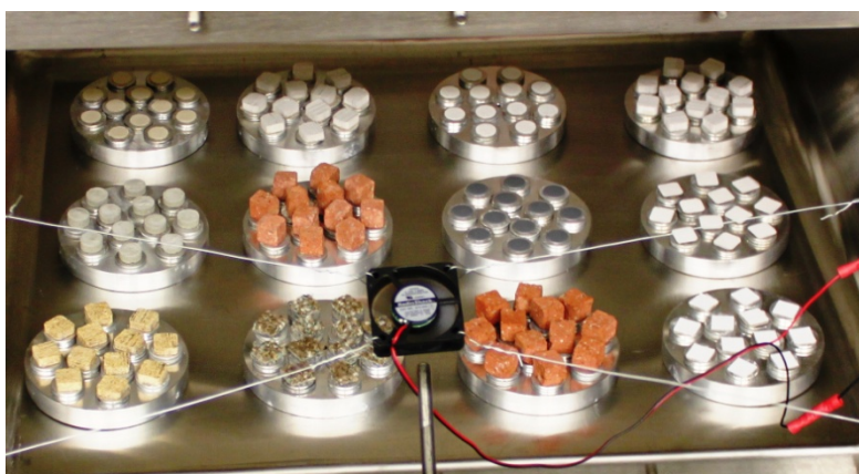
Figure 4.6. Twelve support blocks with sink materials for Test S-3
