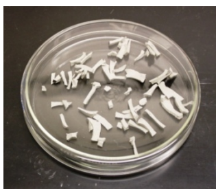
Figure 4.3. Field caulk source containing Aroclor 1254
