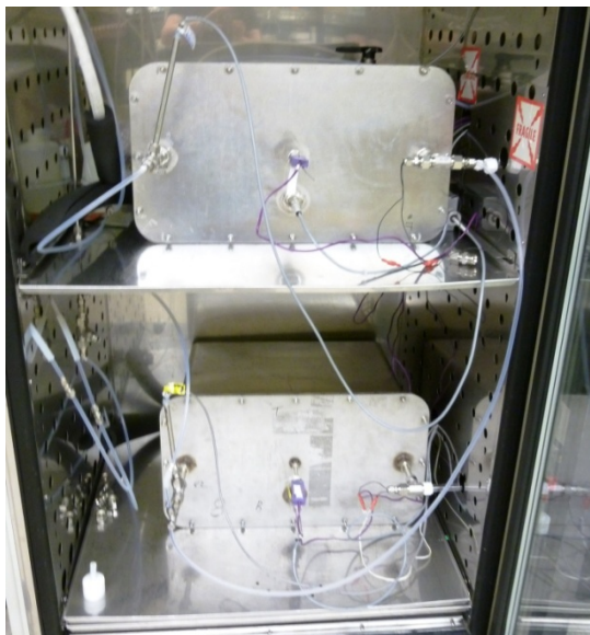
Figure 4.1. Picture of source chamber (top) and test chamber (bottom)
